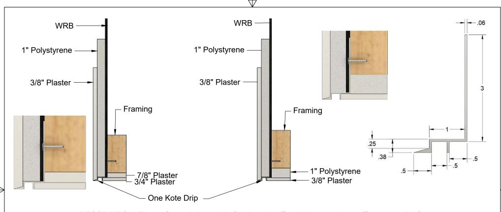
DESCRIPTION: The perfect solution to join fascia and soffits while preventing soffit water stains from runoff. The 1KD One Kote Drip has a 1/2" reveal and accommodates standard One Kote plaster over 1" foam with a 1-3/8" ground. 1KD has a unique feature in that it is weep-able on the fascia.
