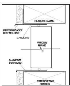
MATERIAL: Aluminum Alloy 6063 T5 ASTM: B 221
