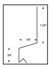
**DESCRIPTION:** The #2 Drip Edge is designed to provide a clean, straight transition between soffit and fascia with an exposed 3/4" surface. The 1/4" x 1/4" angle at the bottom of the trim helps to deflect water from migrating along the soffit.
