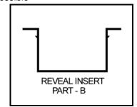
Aluminum Alloy 6063 T5 THICKNESS: Nominal .050 ASTM: B 221 **MATERIAL:**
