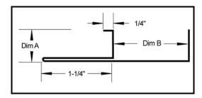
**DESCRIPTION:** Functional reveal that can be used at the wall/soffit joint or when butting to dissimilar
