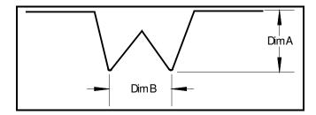
**DESCRIPTION:** Versatile expansion screed used primarily from the corners of exterior door and
