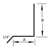
**DESCRIPTION:** The drip edge is used in applications above exterior openings as a termination point
